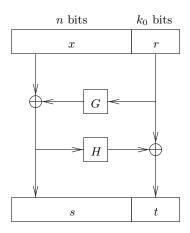
Fig. 1. A diagram of the OAEP
