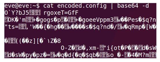
This is because the PVC-2300 uses a non-standard base64 key string, as evidenced by analyzing its encode64 and decode64 functions:
