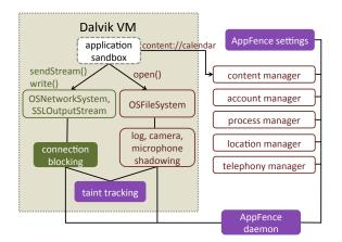
Figure 2: AppFence system architecture. The Dalvik VM sandboxes the application and contains the Android core libraries. Resource managers reside in the Android framework outside of the VMs. Existing resource manager and file system components are modified for shadowing, while exfiltration blocking introduces new components (solid boxes) for connection blocking and taint tracking. The AppFence daemon runs as a native library, and is controlled by the AppFence settings application.
