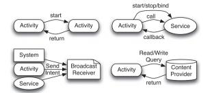
Figure 2. Typical Android application component IPC.
