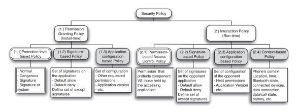
Figure 3. Policy tree illustrating the example policies required by applications. The double-stroke boxes indicate support by the existing platform.
