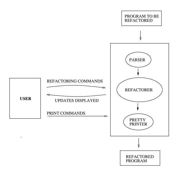
Figure 11.1: Software Refactoring Process
