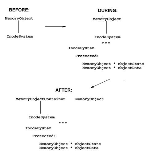
Figure 3.3: Superclass Converted to Component
