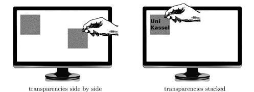
Fig. 1: Example for Visual Cryptography with a Transparency Displayed on a Monitor and a Transparency which is Physically Put in front of the Monitor
