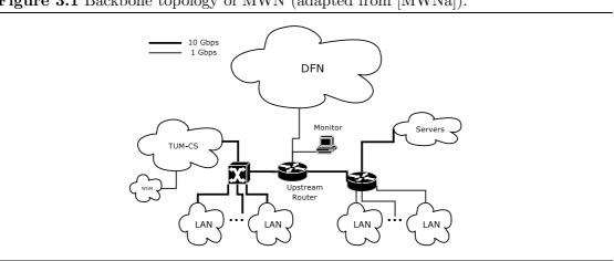
Figure 3.1 Backbone topology of MWN (adapted from [MWNa]).
