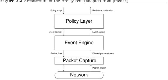
Figure 2.3 Architecture of the Bro system (adapted from [Pax99]).
